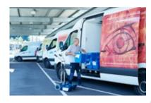
All vehicles GDP-compliant Galexis, Alloga, UFD and Pharmapool each operate their own fleet, which together comprise 158 delivery vans (up to 3.5 tonnes). All vehicles are GDP-compliant and are fitted with an air conditioning system in the loading space, which is mandatory for the transport of pharmaceutical products.
